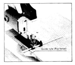
To attach the guide rule (rip fence), use the hex wrench to loosen the bolt on the base in front, slip in the guide rule and secure the bolt.
